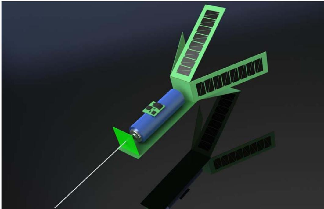
Figure 1.0 CAD Model of Eagle-1—On-orbit configuration with solar panels deployed
